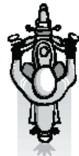
Proper braking. Neither wheel is locked and motorcycle is in alignment.
